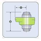
Figure 1002 10,000 psi cwp (690 bar) 1-4" 7,500 psi cwp (483 bar) 5-6"
